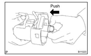
(b) Apply a light coat of gasoline to the O-ring, and push in the pressure regulator.
