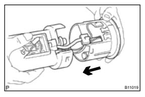
(b) Install the fuel suction plate to the fuel filter and fuel pump assembly.
